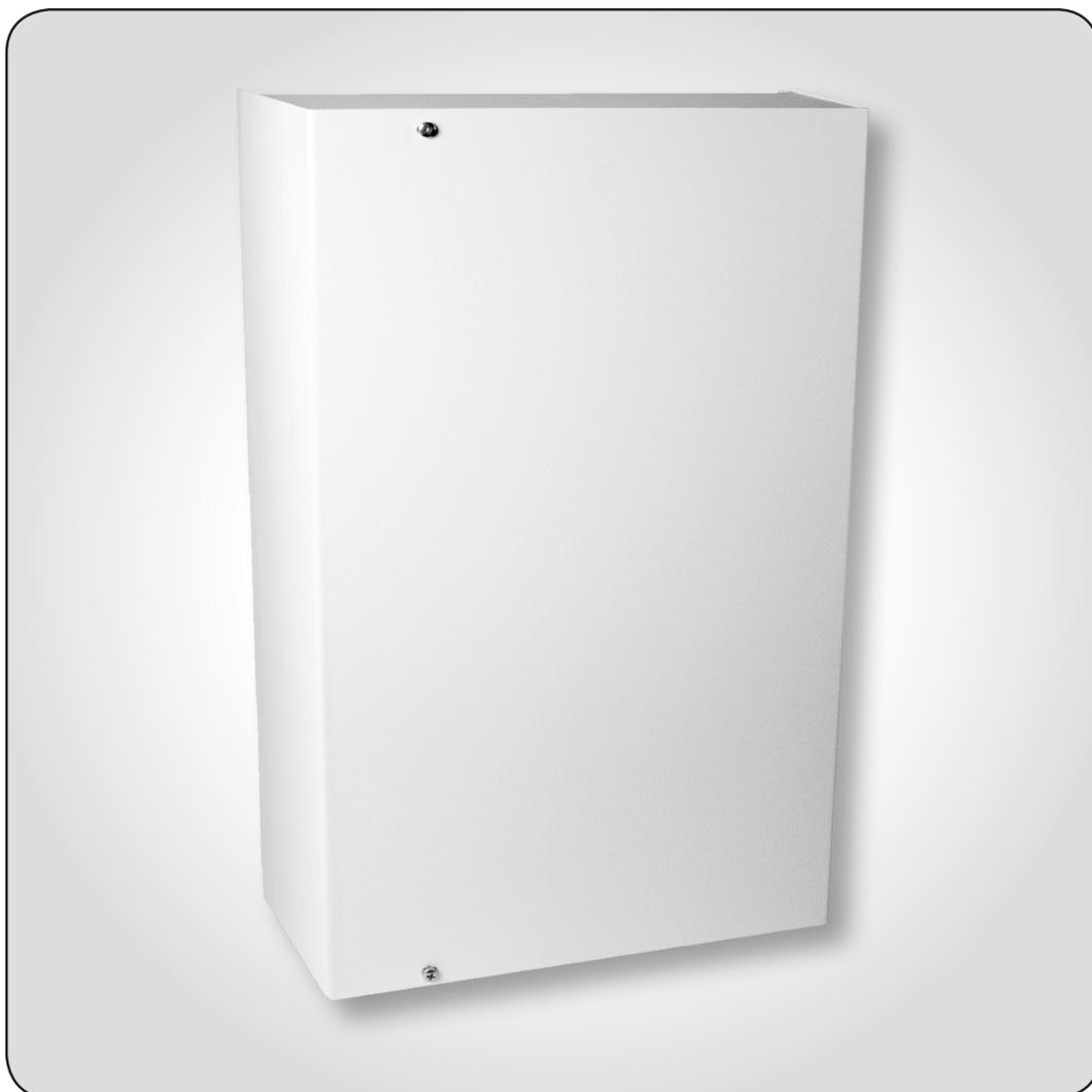
The EL-2 emergency light control panel features two lines, each line can accommodate 127 exit signs, route lights or I/O units. The EL-2 supplies the operational voltage to the light units during normal conditions, whilst also completing the continuous testing and monitoring of the equipment on the system. All monitored event information is saved in the memory of the control panel, and this can be accessed by a connected EL-KP key pad (see page 13).
